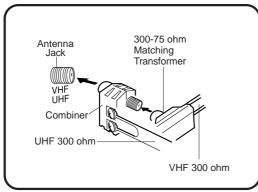
Connect the UHF 300 ohm Twin-lead Wire to the Combiner (not supplied). Connect the VHF 300 ohm Twin-lead Wire to the 300-75 ohm Matching Transformer (not supplied). Attach the Transformer to the combiner, then attach the Combiner to the Antenna Jack.
